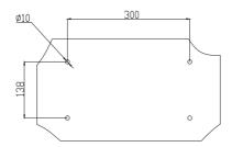
Use M6\*50 screws to fix the Junction box to the wall through the 4 fixing holes at the bottom of the Junction box.
