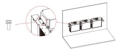
Fixing bracket connecting plate
