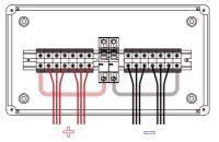
Connect the positive / negative inverter cable to the left / right hole of the MCB respectively.
